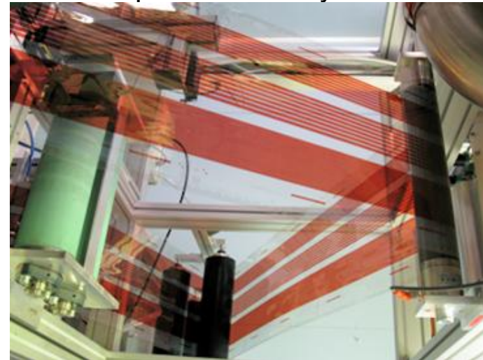
Video of R2R gravure printing of photoactive layer
