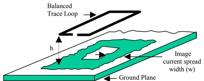
Figure 3. Image current loop formed by a balanced trace.
