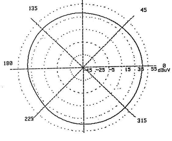
Graph 4B. Balanced Trace above Ground Plane Radiation
