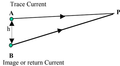
Figure 5. Signal Current Radiation and Image or Return Current Radiation at a Point  $P$  on the Antenna
