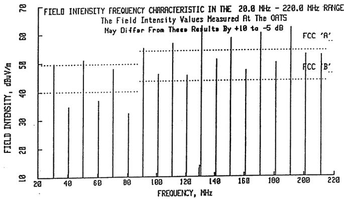
Graph 2B. Balanced Trace above Ground Plane Radiation.
