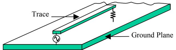
Figure 2. An Unbalanced Trace (Current is Path is through Ground Plane)
