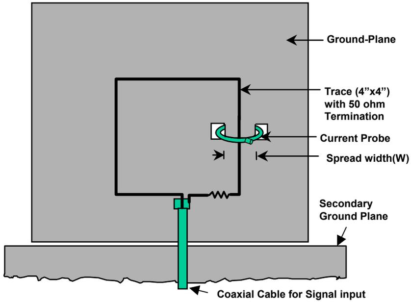
Figure 6. Current Spread Measurement set-up
