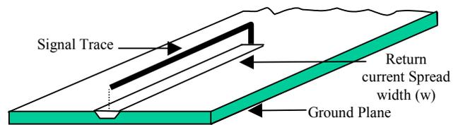
Figure 4. Return current spread of an unbalanced trace
