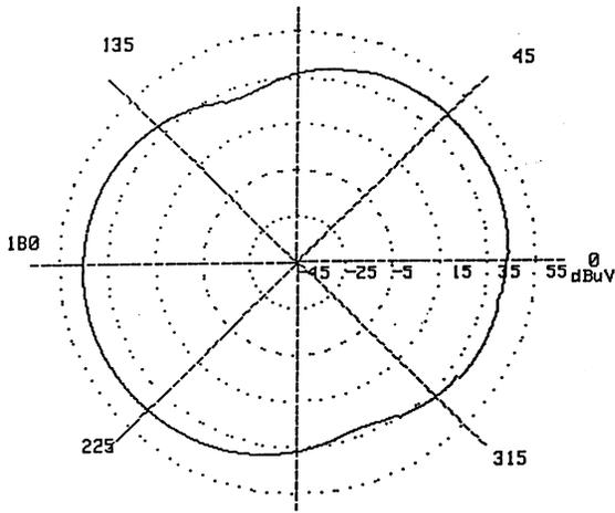
Graph 3B. Balanced Trace above Ground Plane Radiation
