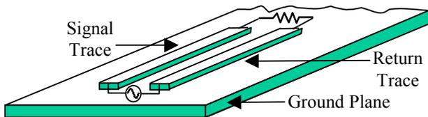
Figure 1. A Balanced Trace circuit loop over a Ground Plane (Ground Plane is isolated from Traces)
