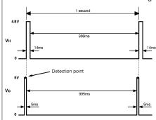
cycle of 1 second. Each VH cycle is comprised by 4.8V being applied to the heater for the first 14ms, followed by 0V pulse for the remaining 986ms. The Vc cycle consists of 0V applied for 995ms, followed by 5.0V for 5ms. For achieving optimal sensing characteristics, the sensor's signal should be measured after the midpoint of the 5ms Vc pulse of 5.0V (for reference, see timing chart below).
