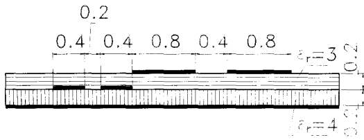
Fig. 3. Sketch of a multiconductor transmission line on a multilayered board. All dimensions are in mm.
