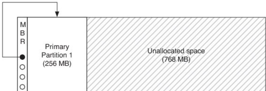
Figure - Device after partition initialization
