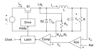
Clock controls turn-on Peak current controls turnoff During the on time,  $I_{S1} = I_{L}$
