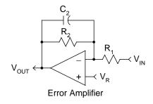
$$K(s) = \frac{-V_{OUT}(s)}{V_{IN}(s)} = \frac{R_2}{R_1(1 + R_2C_2s)}$$
