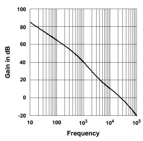
The gain – bandwidth is greater than 25 kHz.
