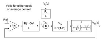
Fig. 35. Flow graph of single-loop linearized c/m controlled boost converter.
