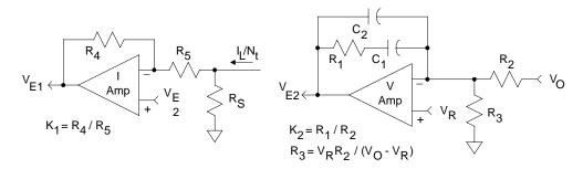
Step 1: Choose  $I_{L(p-p)}R_S/N_t$  so that it is well above the noise level, e.g.  $I_{L(p-p)}R_S/N_t=0.5$  volts.
