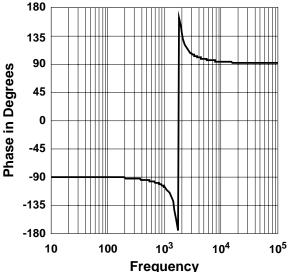
$$\begin{split} \text{Peak} &= \frac{V_i}{2\pi f V_P R_1 C_2} \cdot R \sqrt{\frac{C}{L}} \\ \text{for 6 dB gain marg in at } f = 1.71 \text{kHz}, \\ &\frac{V_i}{2\pi f V_P R_1 C_2} \cdot R \sqrt{\frac{C}{L}} = \frac{1}{2} \Rightarrow R_1 C_2 = 299 \\ \text{Sample values: } R_1 = 167 \text{ k}\Omega, \ C_2 = 0.02 \, \mu\text{F} \end{split}$$
