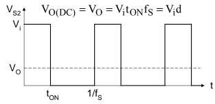
Fig. 6. The buck converter.
