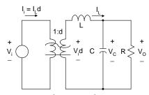
$\begin{aligned} &v_i = V_i + \hat{v}_i \quad i_L = I_L + \hat{i}_L \quad d = D + \hat{d} \quad \text{Neglect "hat" products} \\ &\text{For example, } v_i d \approx (V_i + \hat{v}_i)(D + \hat{d}) = v_i d + V_i \hat{d} \quad \text{where } \hat{V}_i \hat{d} \approx 0 \end{aligned}$
