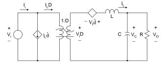
Fig. 11. Linearized buck converter.
