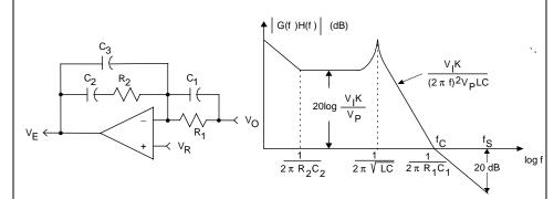
Step 1: Choose gain - bandwidth  $f_C = \frac{f_S}{10}$  for large - signal stability (20 dB attenuation at  $f_S$ ).
