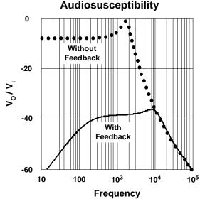
Fig. 21. Output impedance and audiosusceptibility for the lead-compensated sample buck converter.
