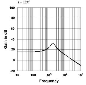
Voltage Loop:  $G_2(s)H_2(s) = \frac{\left(\frac{2\gamma f_S}{1-D}\right)\left(\frac{NtK(s)}{R_SC}\right)}{s^2 + \frac{s}{RC} + \frac{1}{LC}}$
