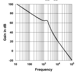
Fig. 24. Individual loop gains for linearized buck converter with peak current-mode control.
