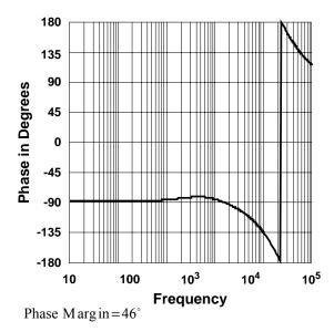
Fig. 37. Open-loop gain function for average current-controlled sample boost converter.
