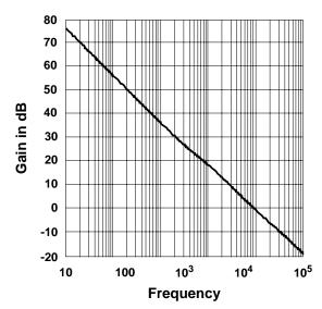
Gain Margin=7dB Gain – Bandwidth>9kHz
