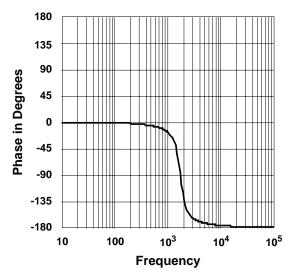
Fig. 14. Bode plot of a 100 W, 12 V-to-5 V, buck converter open loop gain with DC error amp gain  $\lceil K(s) = K \rceil$ .
