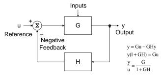
Fig. 4. Flow graph of feedback control.
