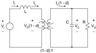
Circuit model using DC transformer concept
