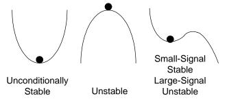
Fig. 2. Large-signal vs. small-signal stability.
