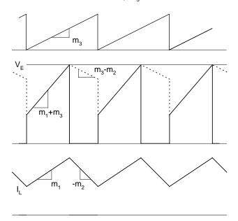
• Effective analog waveform with stabilizing ramp m<sub>3</sub>
