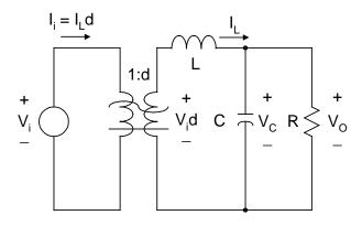
Circuit Model Using DC Transformer Concept. I<sub>L</sub>d and V<sub>i</sub>d are nonlinear terms.
