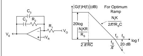
$$\begin{split} \text{Step 1: Choose } & R_S/N_t \text{ so that the effective peak - to - peak current analog (including ramp)} \\ & \frac{R_SD(V_i+V_O\,/\,2)}{N_tf_SL} \text{ is well above the noise level, e.g. } 0.5 \text{ volts.} \end{split}$$
