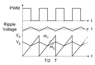
Fig. 19. Large-signal stability considerations for voltage-mode control.
