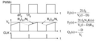
Fig. 22. Peak current-mode control implementation for buck converter.
