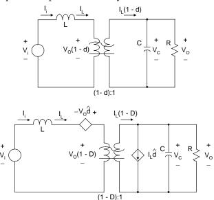
Fig. 29. Linearized boost converter.
