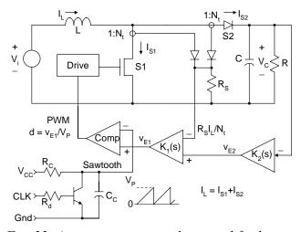
Fig. 33. Average current-mode control for boost converter.
