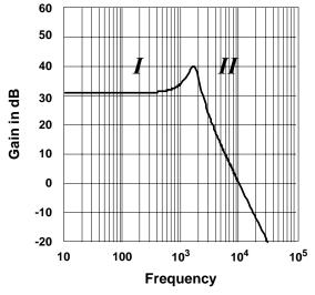
$$Peak = \frac{V_i K}{V_P} \bullet R \sqrt{\frac{C}{L}} = 40 dB \ at \ 1.71 kHz$$
