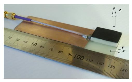
Low- Profile 17.0x25.0x5.0mm. Design for use with no ground beneath the antenna
