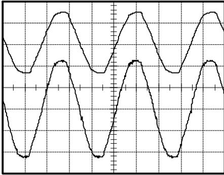
Fig. 12. Waveforms of phase voltage and current at full load. Horizontal scale, 5ms/div. Top: input phase voltage 100V/div. Bottom: input phase A current, 2A/div.
