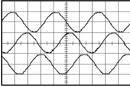
Fig. 11. Three phase inductor current waveforms at full load. Horizontal scale: 5ms/div; vertical scale, 5A/div.
