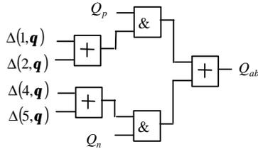
Fig. 9. Realization of control signal for switch  $S_{ab}$ .
