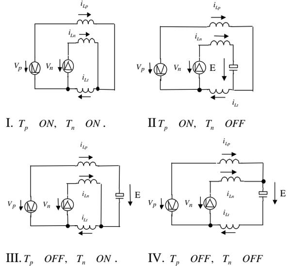
Fig. 4. The equivalent circuits for the parallel-connected dual-boost topology in all four switching states.
