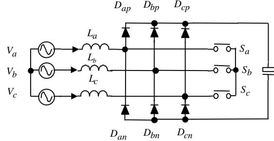
(b). 3-phase boost rectifier with star-connected  $3f$  switches.
