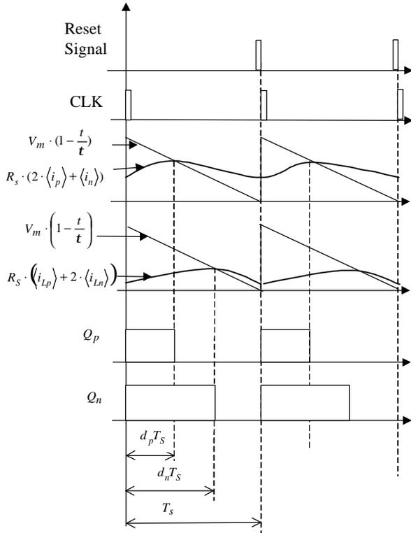
Fig. 8. The waveforms of the control core in Fig. 6.
