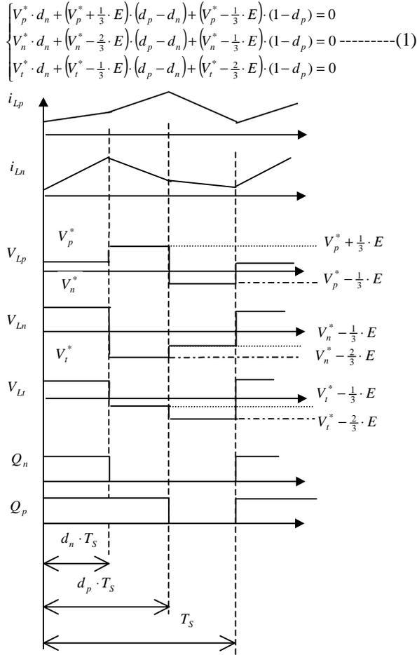
Fig. 5. The inductor voltage and current waveforms for the topology shown in Fig. 3 (a) under the condition  $d_p > d_n$ .
