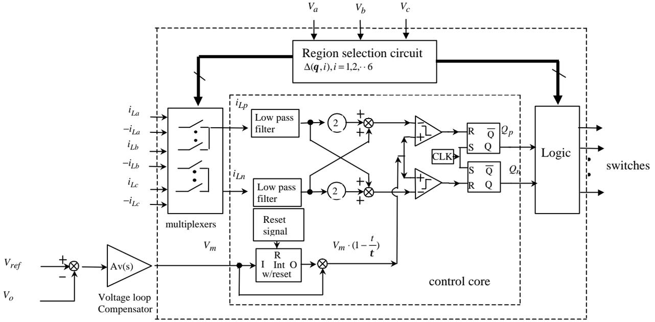
Fig. 6. The control block of the proposed general three-phase PFC controller-I
