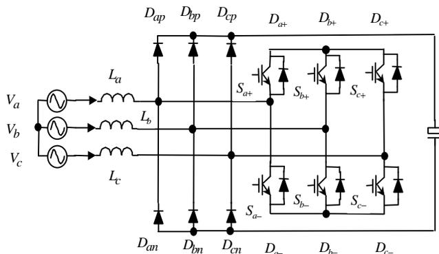
(e). 3-phase boost rectifier with an inverter network
