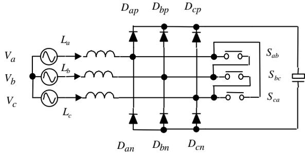
(a). 3-phase boost rectifier with delta-connected  $3f$  switches.
