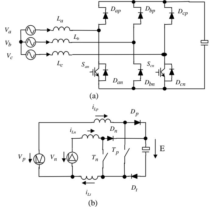
Fig. 13. The three-phase H bridge boost rectifier (a). The equivalent circuit for interval 0~60°. (b). The parallel-connected dual-boost topology.
