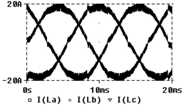
Fig. 14. Simulated current waveforms for three-phase H bridge boost rectifiers shown in Fig. 1 (c) and (d) with proposed general three-phase PFC controller.
