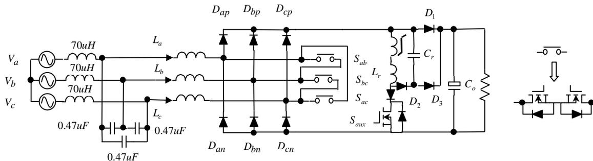
Fig. 10. The schematic of experimental three-phase boost PFC with active soft switching.
