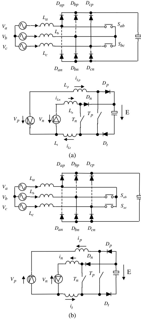
Fig. 3. The equivalent circuit of 3-phase boost rectifier with delta-connected switches and its corresponding parallel-connected dual-boost topology. (a) (0~60°). (b). (60°~120°).
