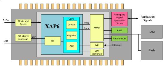
XAP6 is a 32-bit processor IP core available as Verilog RTL. It offers advanced computing functions at the lowest possible cost and energy consumption.
