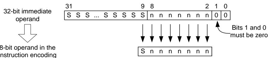
This encoding can therefore represent immediates in the range -512, -508, ..., +504, +508. Immediates outside this range require an alternative encoding of the instruction.
