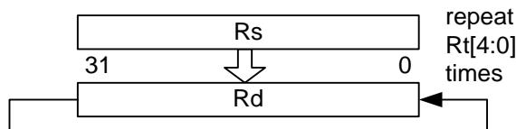
**Usage Notes**      The rotation is a 32-bit rotation and does not rotate through the carry bit.
