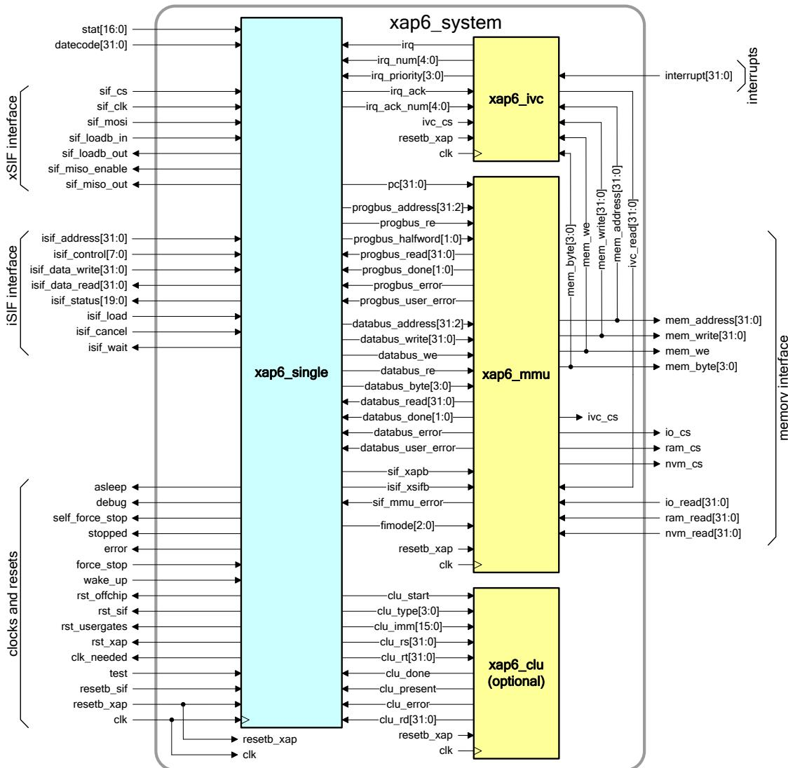
The XAP6 can address 4GB of linear memory space, normally populated with a mixture of Flash, RAM and I/O registers. Code and data can exist in the same memory.
