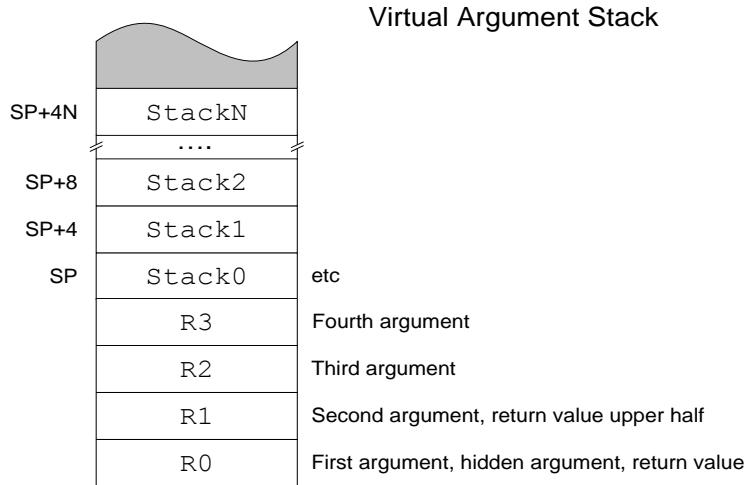
The rest of the virtual argument stack is held in the XAP6's physical stack in memory. While it is slower to access than registers, space on the physical stack can be dynamically allocated and freed at runtime simply by pushing and popping values on and off the stack.
