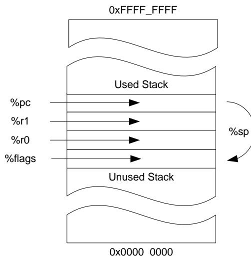
A Soft Reset will take place if a Context Push is made before the required stack is initialised.
